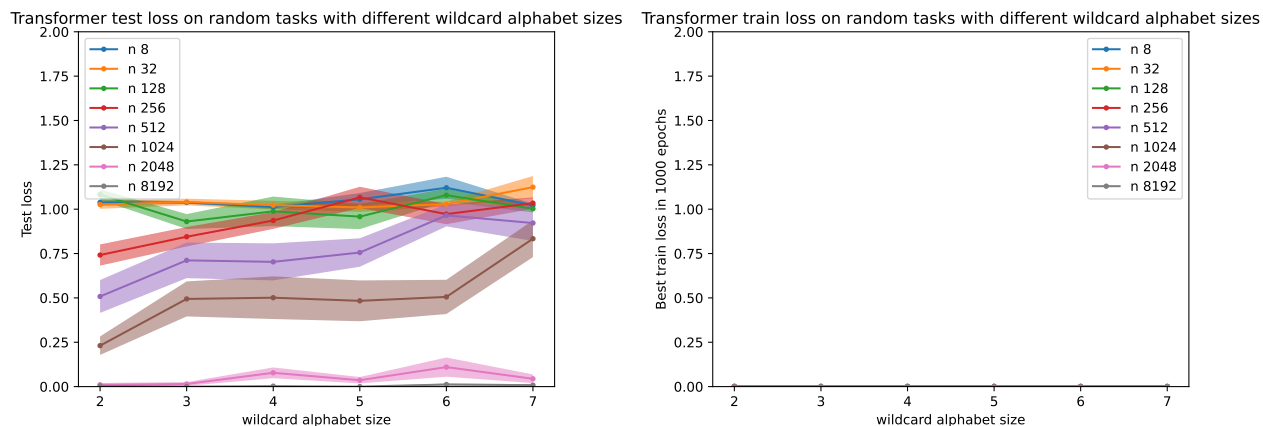
Figure 18: Performance on tasks corresponding of two random templates of length 5, labeled with 1, -1, respectively. Each template is sampled randomly from \mathcal{W}^5 , conditioned on the two templates being distinct. We vary the wildcard alphabet size |\mathcal{W}| . Performance generally degrades as the wildcard alphabet size increases.
